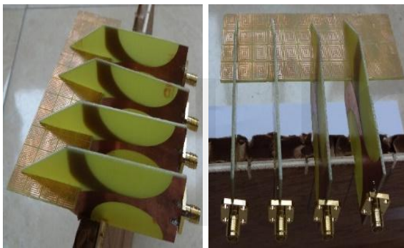
Fig. 16 Photograph of the fabricated antenna array.
